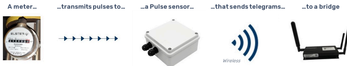
Basic functionality of the pulse sensor
