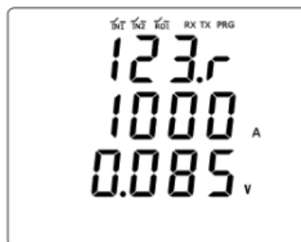
Example of the current transformer ratio configuration menu
